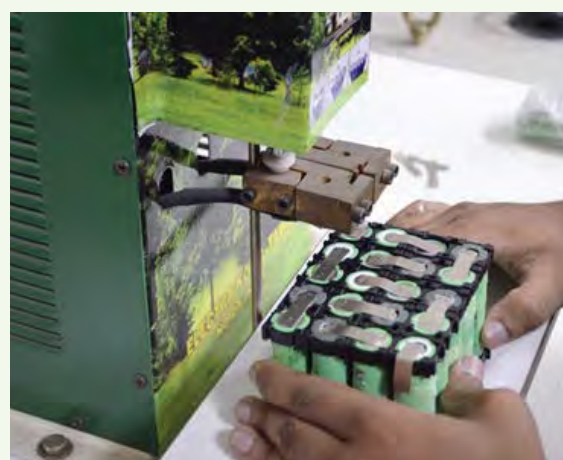
Battery Spot Welding System
