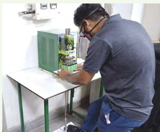
Battery Spot Welding System
