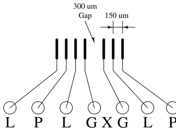
2. Each power (P) signal should have a capacitance of about 2 nF to ground.
