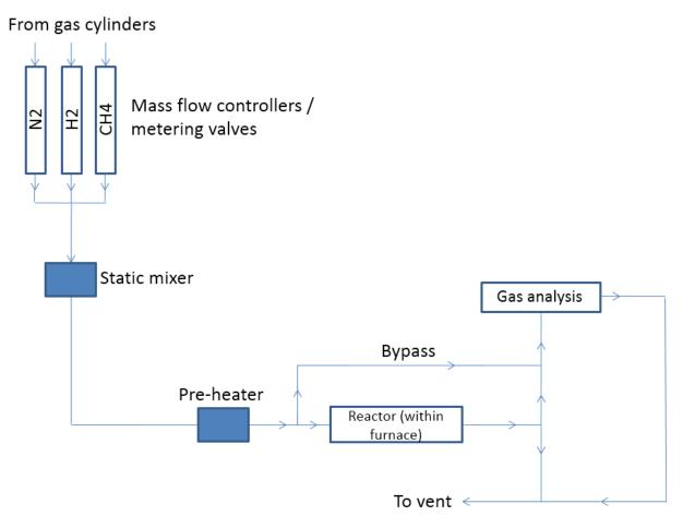
Gas analysis (using gas chromatography) is not in scope of the current tender. Only the connections needs to be provided
