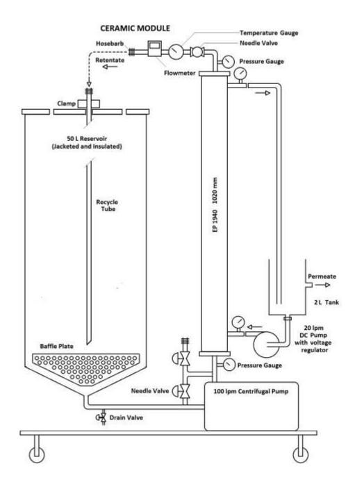
Figure 1: Microfiltration Device (Quantity:1)
