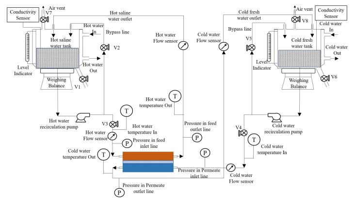
The flow sensors should be placed within ten times of diameter of the feed pipe in upstream side and on the downstream side within the five times of diameter of permeate side.
