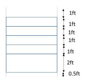
Approx. 37 sq.ft. x 6 shelfs, height adjustable. Specimen will be Max 80% of ft covering 80% area Bottom rack has to be stronger assuming 2500kg/m<sup>3</sup> Dismantalable
