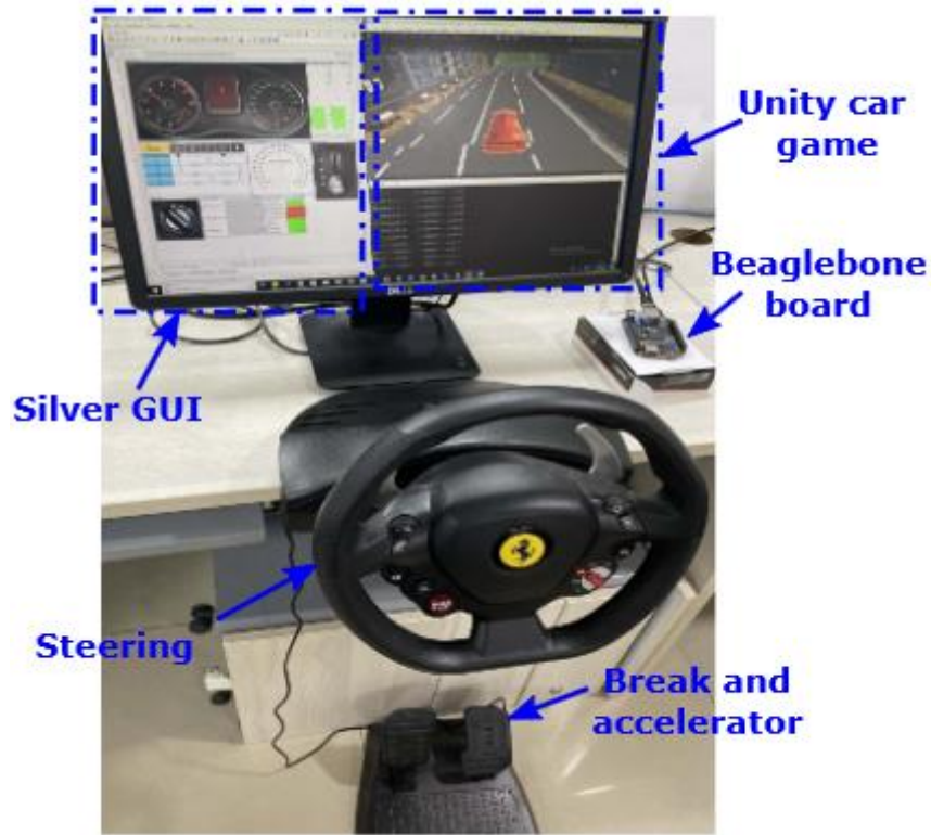
Figure 10: A demonstration of the system. The Synopsys Silver tool generates the CAN bus traces. The Unity simulator is used to drive the car. Note the Beaglebone board that runs the online compression algorithm.
